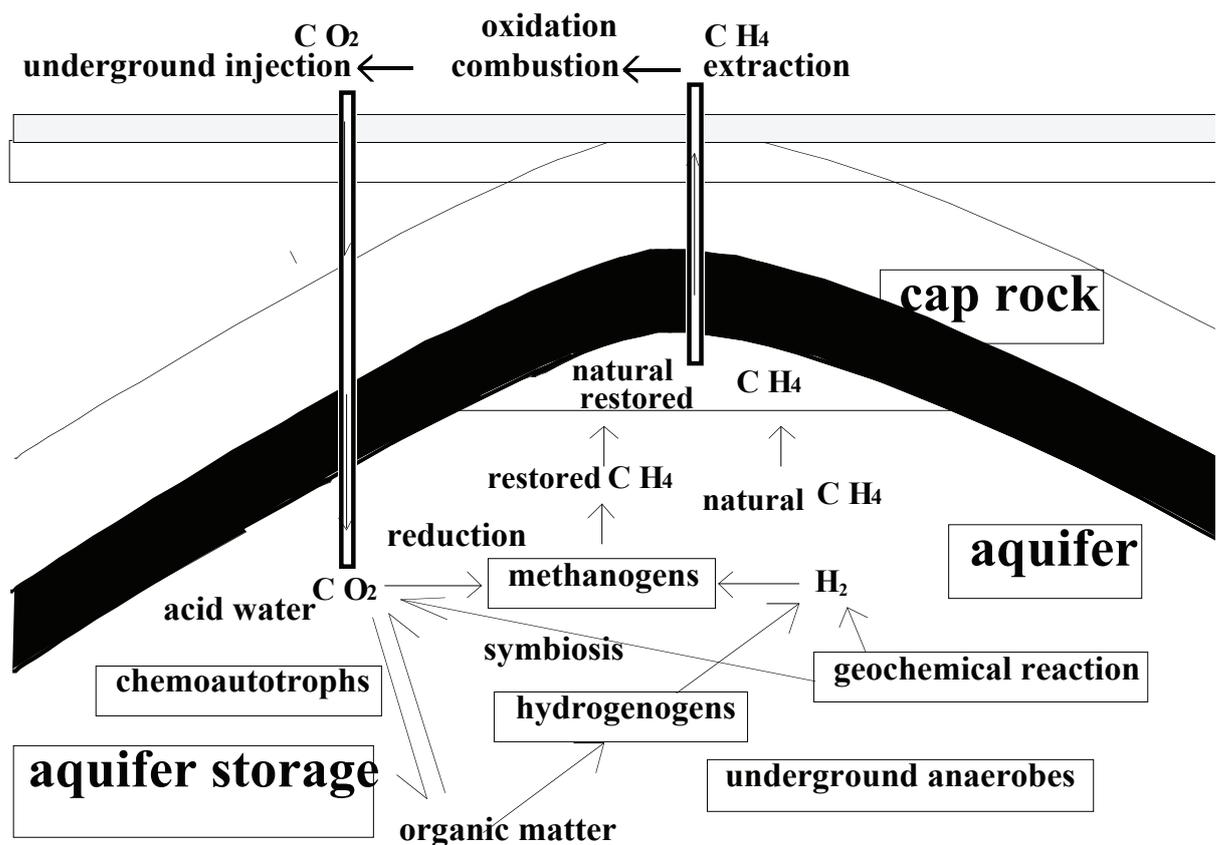
**Fig.3 Geological sequestration of CO<sub>2</sub> and microbial restoration of methane deposit.**
