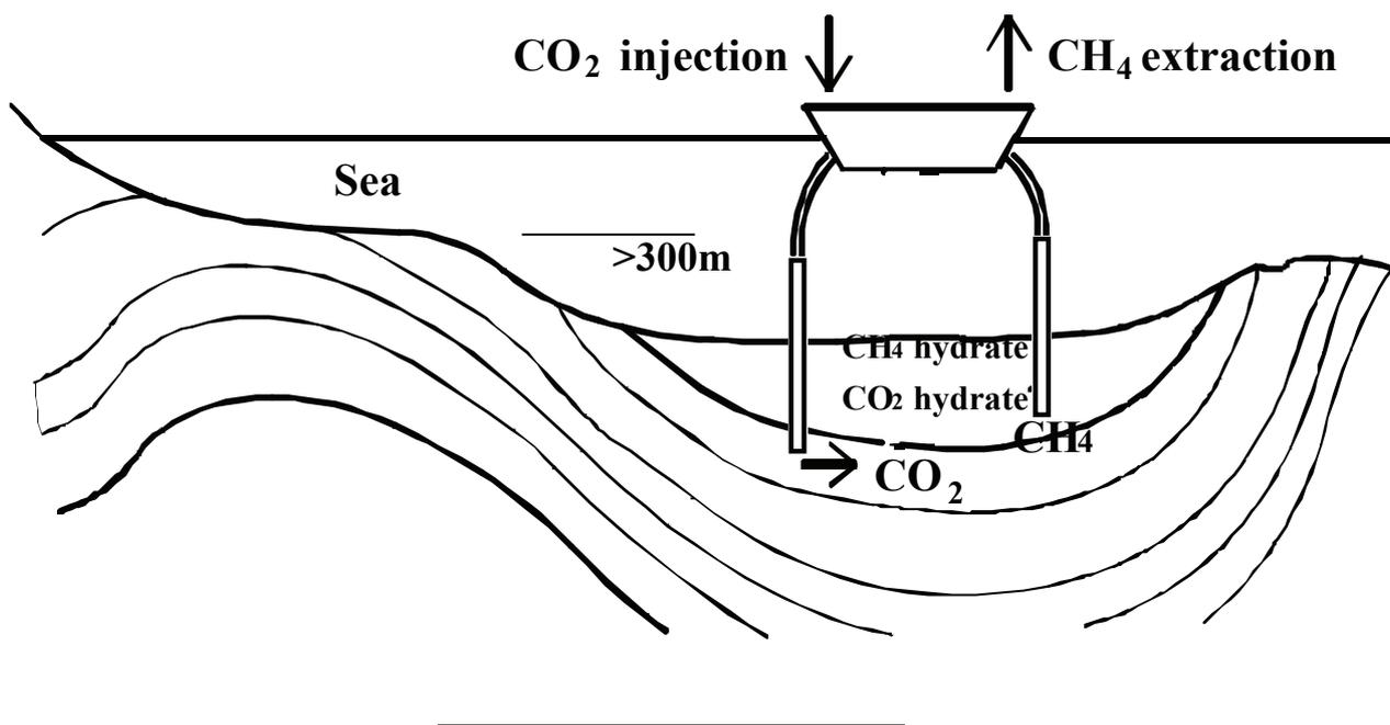
**Fig.2 Injection of CO<sub>2</sub> under methane hydrate layer and extraction of methane.**
